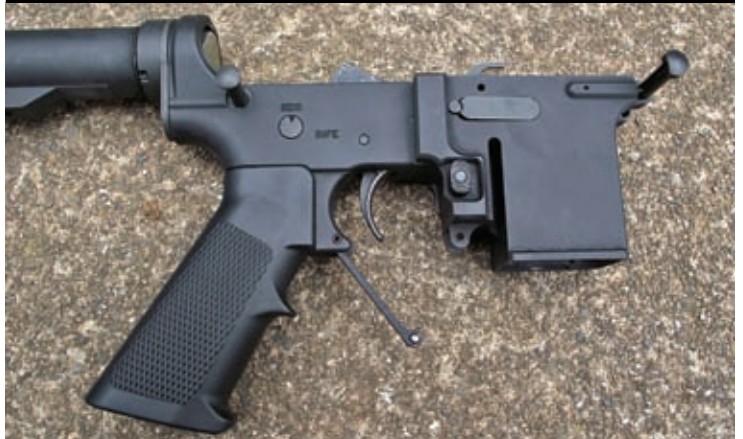
Shown left is the triggerguard released, and above it is the lower receiver, sans any mag well. Mag wells simply slide into the groove on the lower receiver and lock in place — only takes a few seconds. Shown below, is the Hydra with the Grease Gun mag well attached to the lower receiver. To remove the mag well, simply unhinge the triggerguard, and press the mag release button, and the mag well slides right off.
