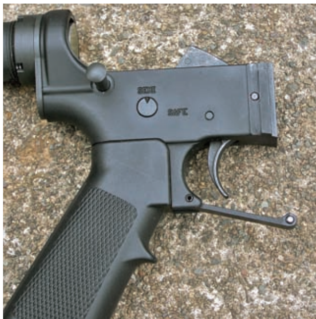
Shown left is the triggerguard released, and above it is the lower receiver, sans any mag well. Mag wells simply slide into the groove on the lower receiver and lock in place — only takes a few seconds. Shown below, is the Hydra with the Grease Gun mag well attached to the lower receiver. To remove the mag well, simply unhinge the triggerguard, and press the mag release button, and the mag well slides right off.
