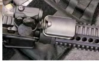
Snap the upper onto the lower receiver as you would a standard AR-15.
