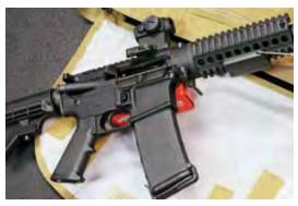
With the bolt locked back and the barrel retaining levers rotated 90 degrees, slide the barrel into the receiver making sure the gas tube lines up properly.
