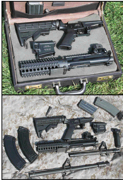
Above: Due to the design of the Modular Weapon System, it breaks down and fits in an extremely small package. All the parts in this briefcase are laid out in the photo below it.
